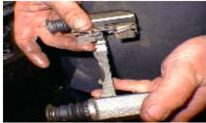
7. Place pad clips on bracket.
