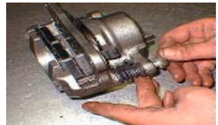
12. Attach bolt thru caliper to attach caliper to bracket.
