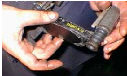
8. Insert pads (with shims already on) into bracket.
