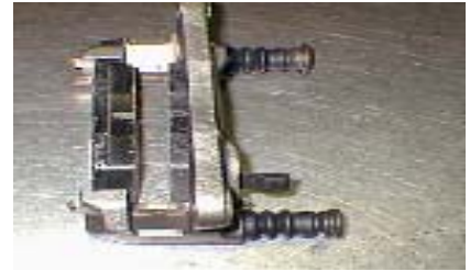
9. Bracket should look like this. Make sure shims are facing out.
