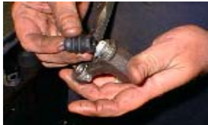
5. Insert rubber bushing over end of bracket.
