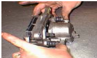
11. Compress guide pins and insert caliper.
