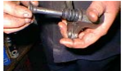
6. Insert guide pin thru bushing so big end will face the caliper.
