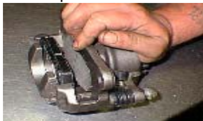
13. Spread pads to allow wide opening for rotor.
