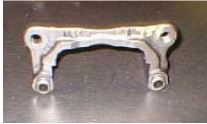
2. Grab correct bracket, don't forget, some units have a left and right hand bracket.
